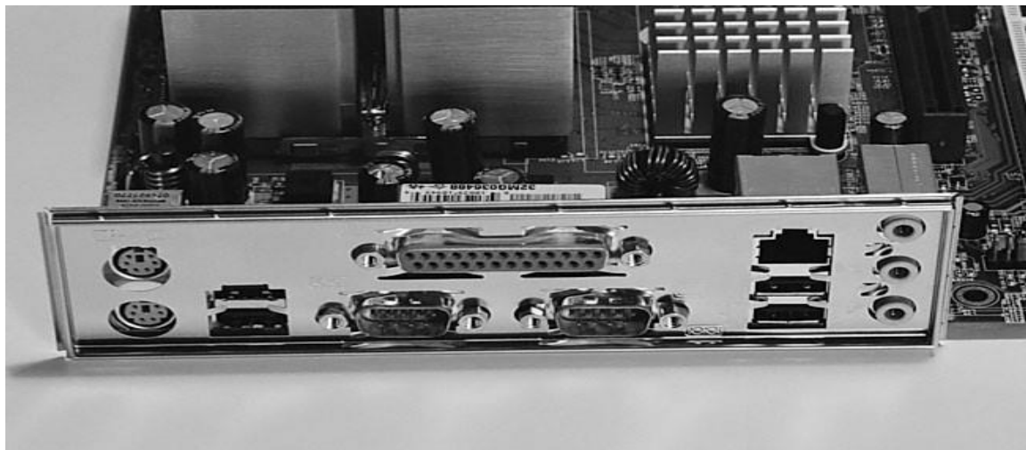
The main board sits behind the I/O shield
