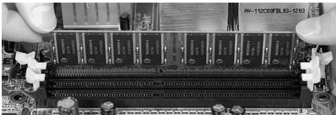
Inserting the memory chip into its slot
